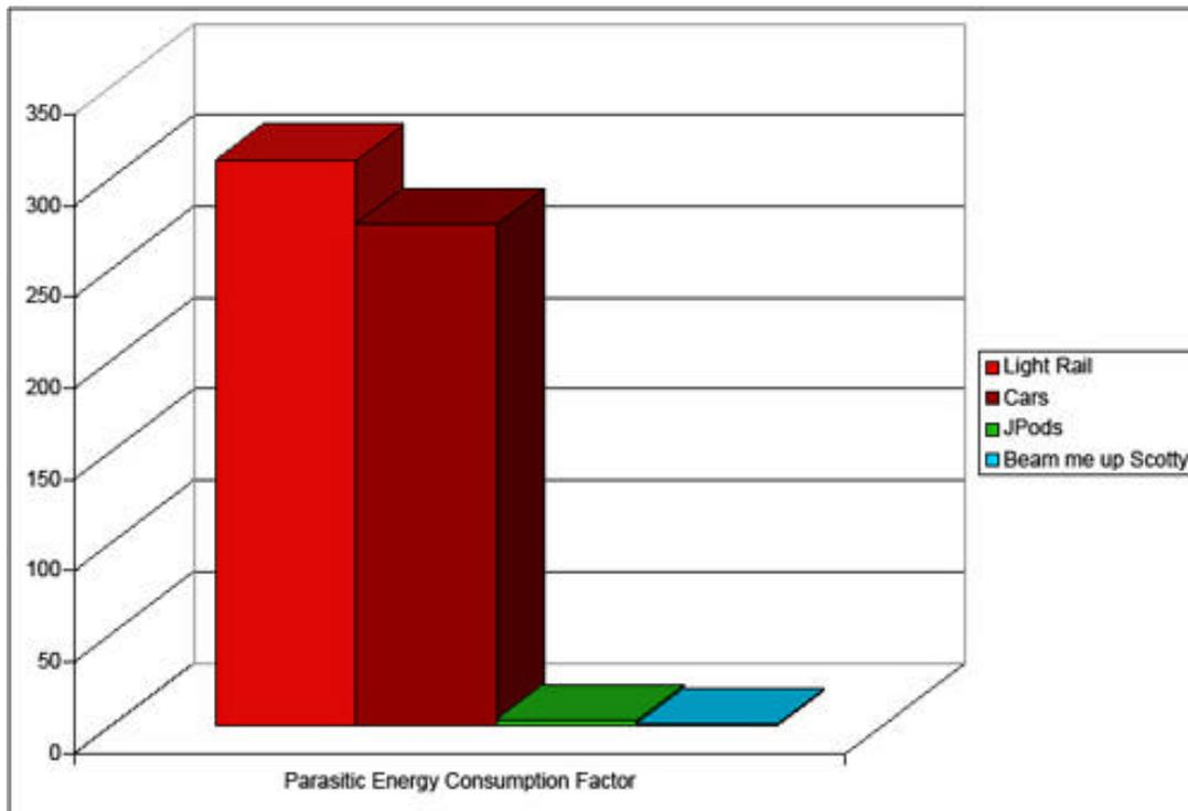
A PEC of 3.25 is possible. JPods are ultra-light computer controlled vehicles suspended from rails that move people and cargo non-stop from origin to destination. A 450 lb vehicle moves a 200 lb person from point of origin to point of destination.
